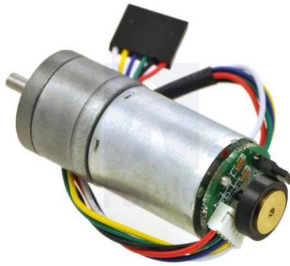
Figure 4. Pololu low power 12V metal gearmotor with 99:1 gear reduction and encoder
