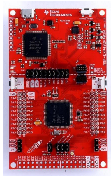
Figure 8. MSP432P401R Launchpad Development Kit Bridge Structural Health Measurement
